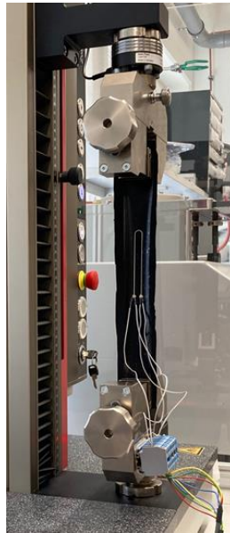
Figure 2: Example of realized textile integrated breath sensor (left), Zwick / Roell equipment of cyclic tensile characterization (right)
