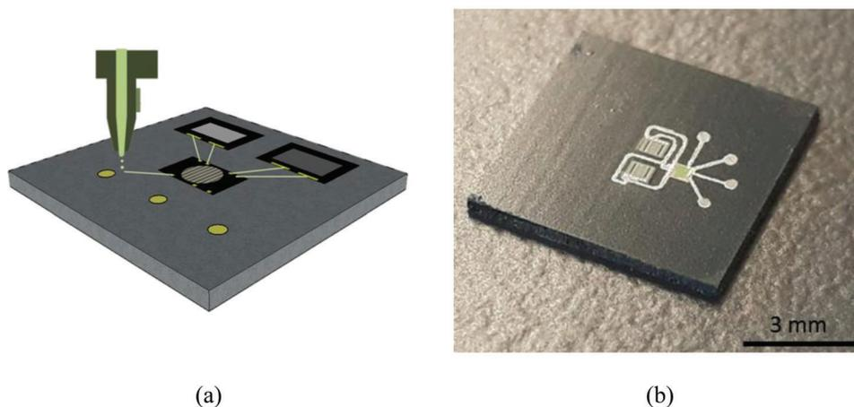
**Figure 27.** a) Schematic illustration of inkjet-printed redistribution layers and via filling for fan-out wafer level packaging. b) Fan-out wafer level packaging of two pressure sensors and application-specific integrated circuit with inkjet-printed redistribution layers.<sup>[19]</sup>
