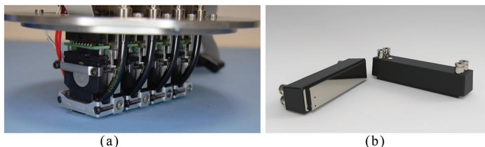
**Figure 4.** a) Multi-printhead array modification to the PixDro LP50;<sup>[86]</sup> b) UHV print engine manufactured by Quantica<sup>[87]</sup> (Reproduced with permission from Quantica).
