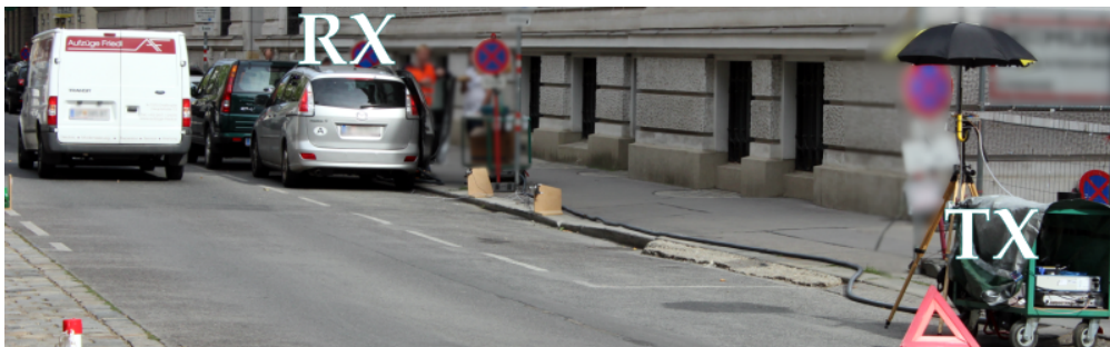
Figure 4. Photograph of the measurement site. The transmitter and receiver are static and urban street traffic is driving by.
